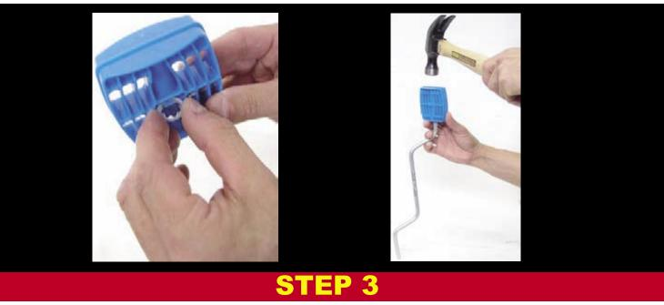
Center the washer in the pedal slot.
