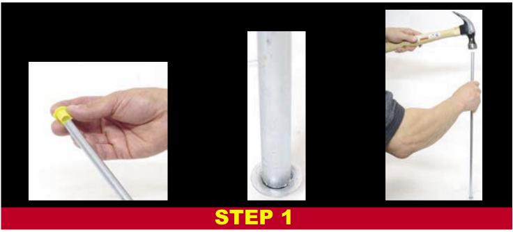
Remove plastic caps on ends of rear axle and discard. *They are for shipping purposes only.*Place one metal capnut on a hard surface with the open side up.
