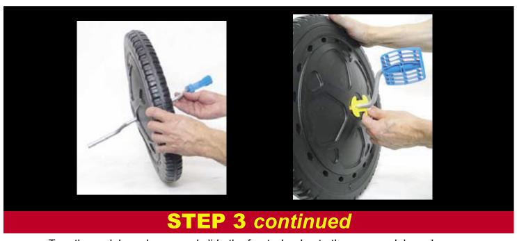
Turn the pedal crank over and slide the front wheel onto the open pedal crank arm.
